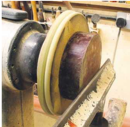
▲ Pic.2 The blank is about 150mm by 40mm. He glued it to his MDF faceplate with hot glue, opting for this method because he didn't want any holes in the top surface
